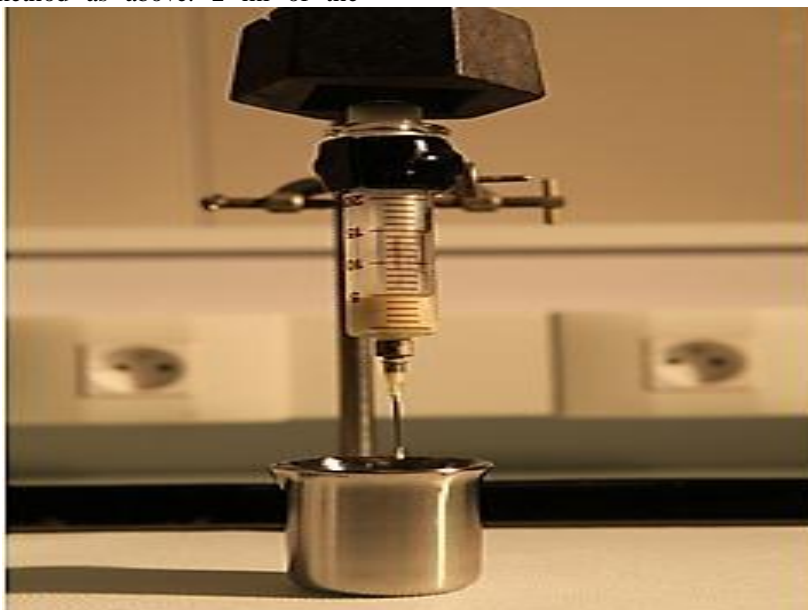
Fig1: Syringeability test apparatus
