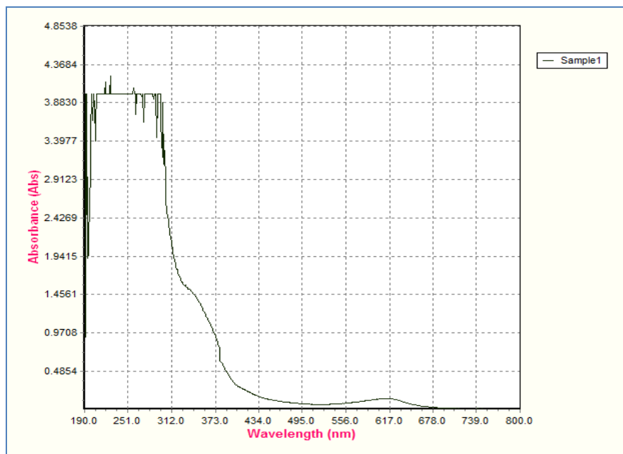
Figure 6: Absorption spectrum of phycocyanin from D20 extraction
