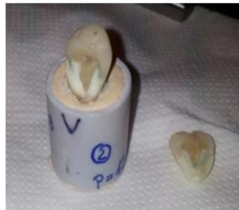
Figure 4. Typical fracture of a specimen from group B after the test.
