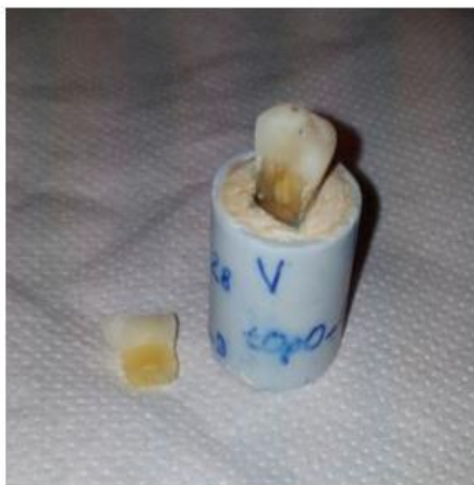
Figure 3. Typical fracture of a specimen from group A after the test.
