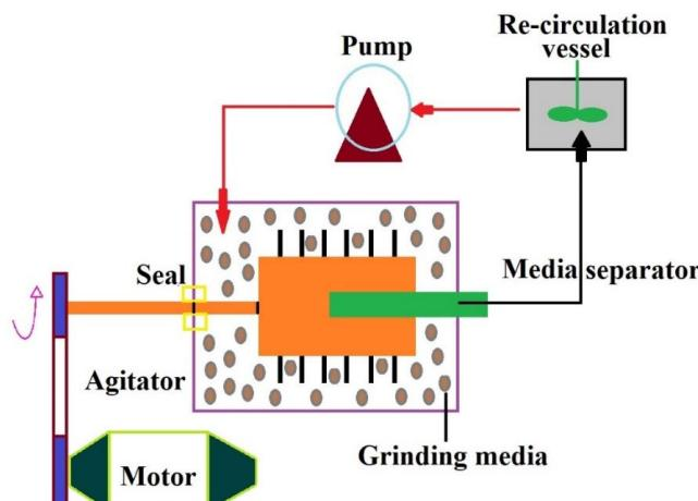
Fig. 2: Schematic representation simplified scheme of a ball milling technology
