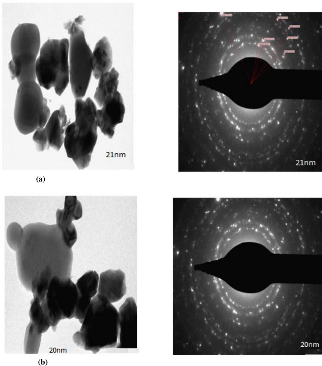
**Fig.3: TEM images with corresponding SAED patterns of the (a)  $\text{CuFe}_2\text{O}_4$  (b) Ag doped  $\text{CuFe}_2\text{O}_4$**
