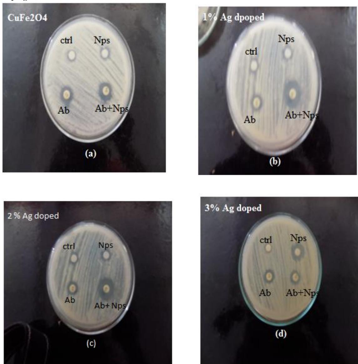
Fig. 6: Zone of inhibition of the antifungal activity of (a) CuFe<sub>2</sub>O<sub>4</sub>, (b) 1% doped Ag, (c) 2% doped Ag, (d) 3% doped Ag powder for Aspergillus Flaves.
