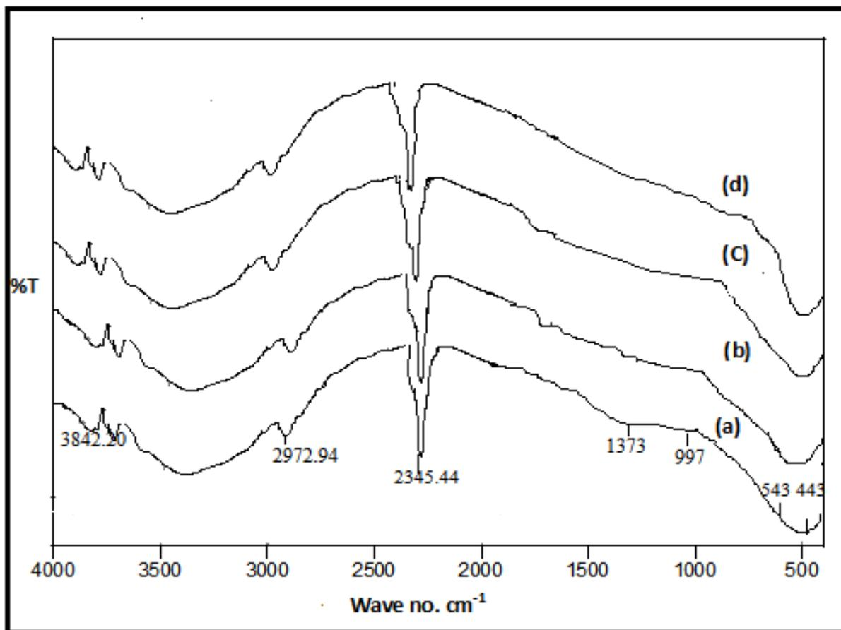
**Fig.2: FTIR Spectra for (a) CuFe<sub>2</sub>O<sub>4</sub> (b) 1% Ag doped CuFe<sub>2</sub>O<sub>4</sub> (c) 2% Ag doped CuFe<sub>2</sub>O<sub>4</sub> (d) 3% Ag doped CuFe<sub>2</sub>O<sub>4</sub> powders annealed at 350 °C.**
