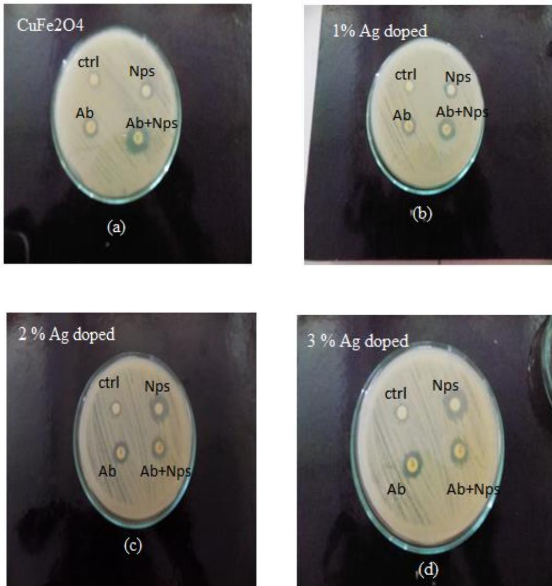
**Fig. 4:** Zone of inhibition of the antifungal activity of (a)  $\text{CuFe}_2\text{O}_4$ , (b) 1% doped Ag, (c) 2% doped Ag, (d) 3% doped Ag powder for *Candida Albicans*
