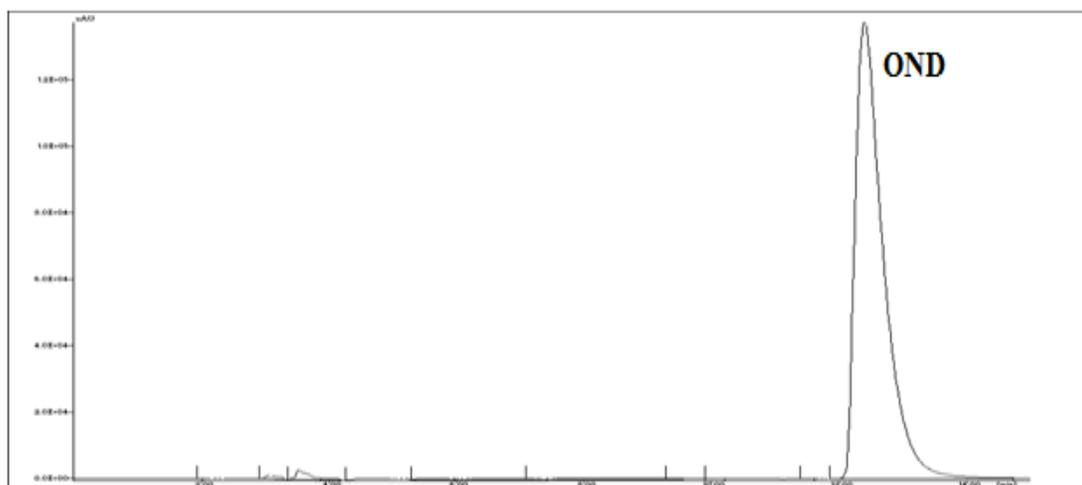
**Fig. 6: Chromatogram of OND HCl after UV illumination exposure**
