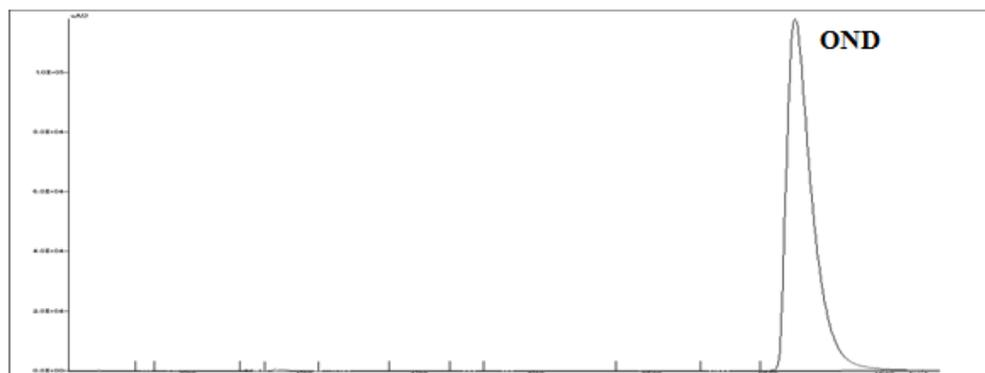
Fig. 5: Chromatogram of OND HCl after dry heat degradation.
