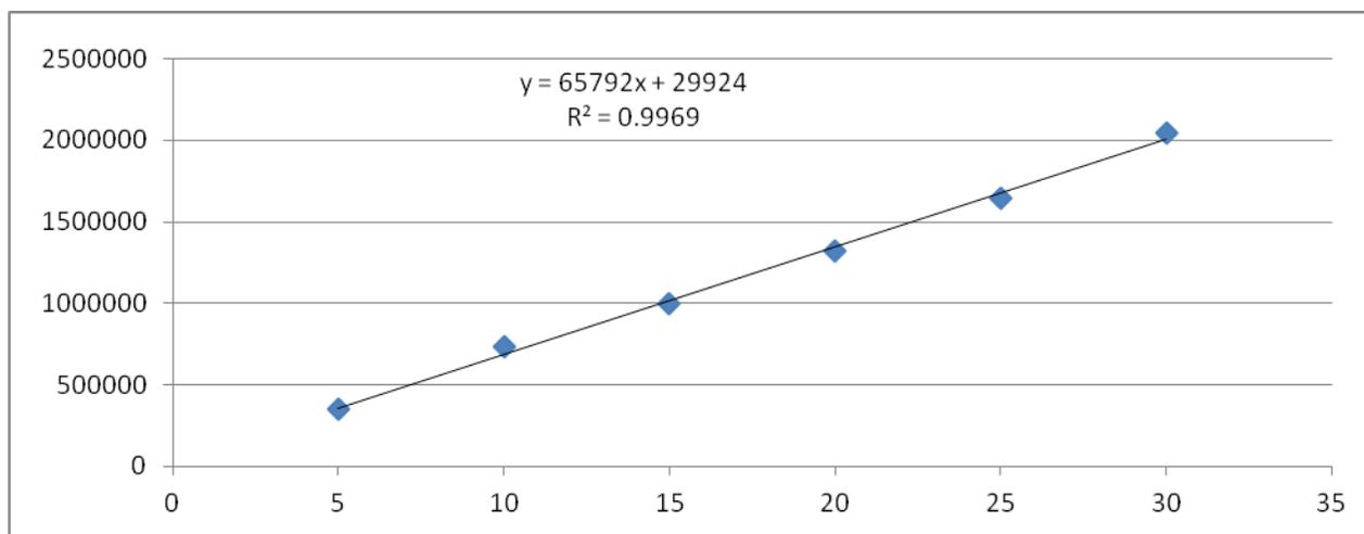
**Fig.8: Linearity curve of Ondansetron HCl (5-30 µg/ml)**
