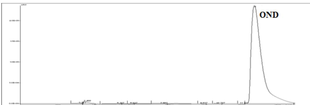
Fig. 2: Chromatogram of OND HCl after alkaline degradation.
