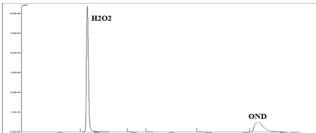
Fig. 4: Chromatogram of OND HCl after oxidation with 30% v/v H<sub>2</sub>O<sub>2</sub>
