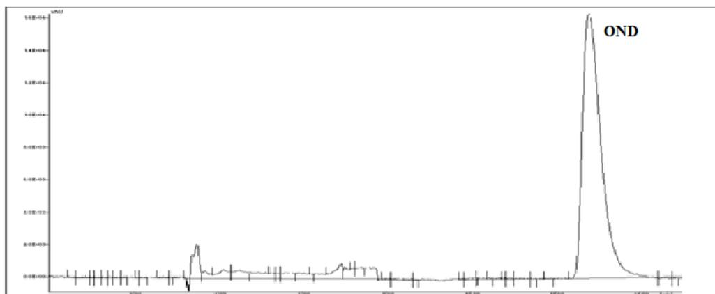
Fig. 3: Chromatogram of OND HCl after acid degradation.
