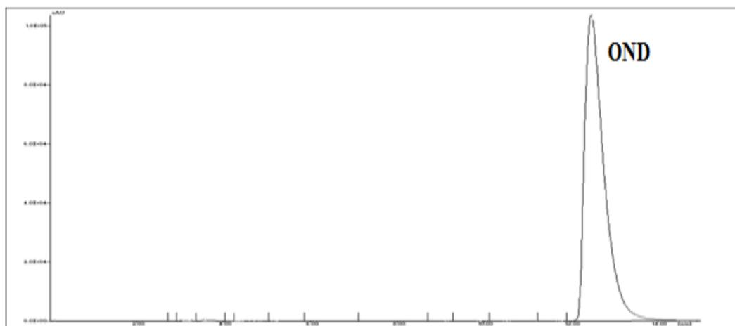
**Fig. 7: Chromatogram of OND HCl after fluroscent light exposure**
