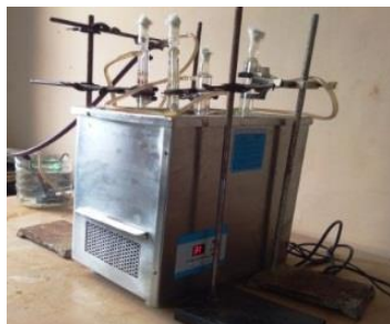
Fig. 1: Ultrasonic irradiator with condense unit
