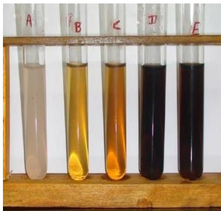
Fig. 1: Color changes during nanoparticles AgNP synthesis
