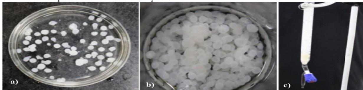
(A, B) Calcium alginate beads, (C) Calcium alginate beads in column
