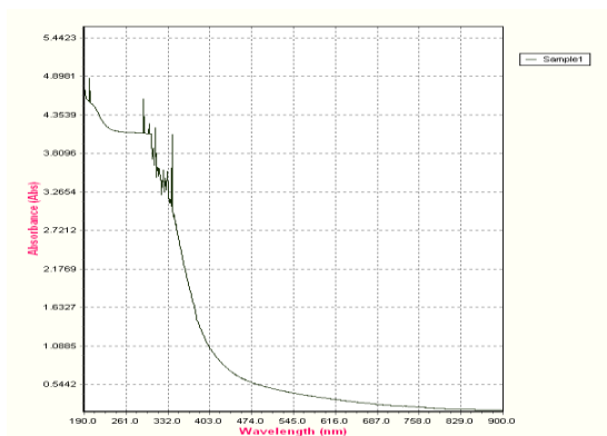
Fig 6: UV-visible spectra of CHE of Vitex negundo Linn plant leaves
