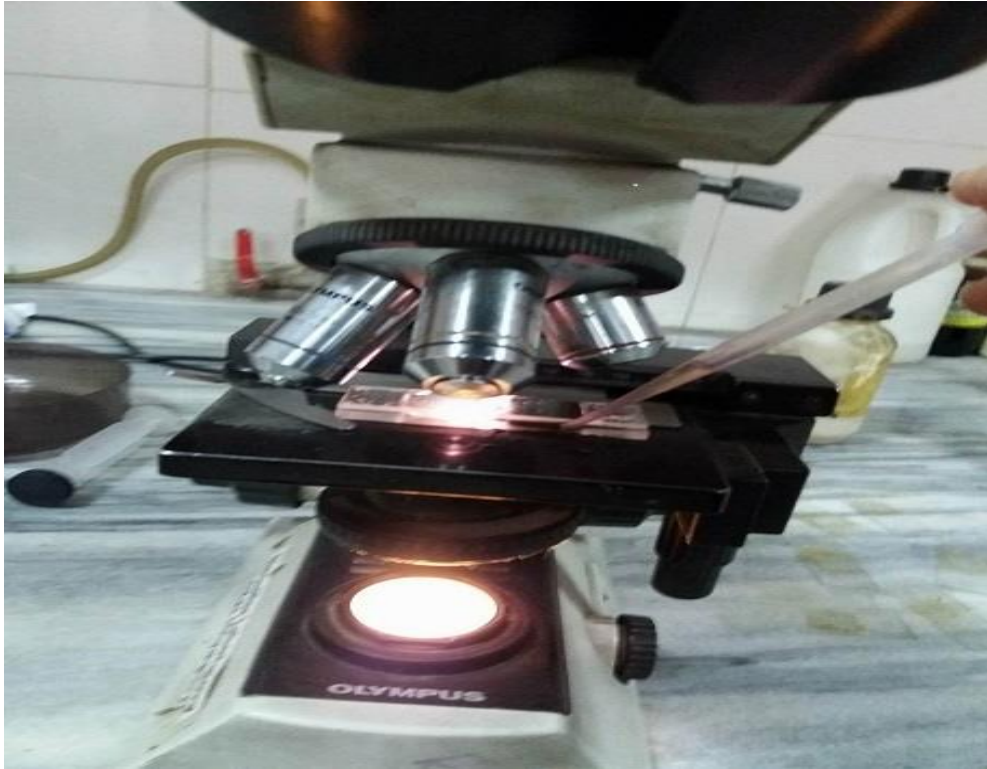
Figure 3.2.2 Filling of McMaster slide.
