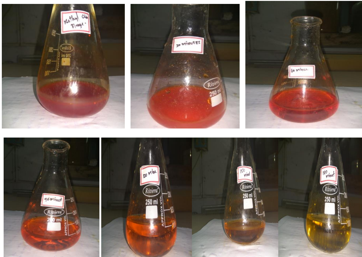
Fig. 10: Color change of methyl orange dye after addition of silver nano particles.
