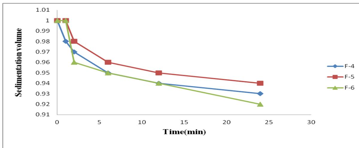
**Fig. 9: Sedimentation volume of formulations using sodium alginate as suspending agent**
