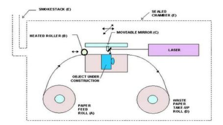
Fig 6: Laminating Object Manufacturing Source: http://www.livescience.com/40310-laminated-object-manufacturing.html
