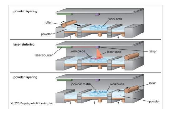
Fig 5: Selective Laser Sintering Process
