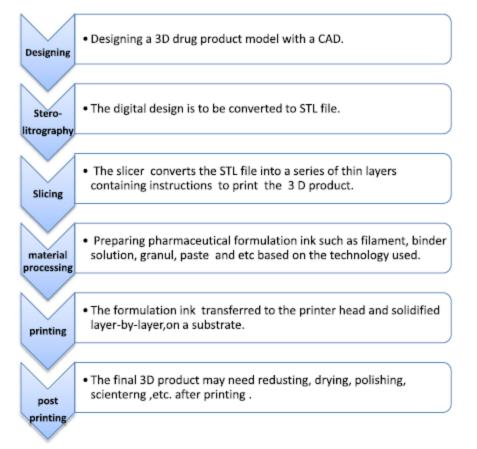
Fig 2: A schematic representation of different processing steps involved in fabrication of 3D printing objects.
