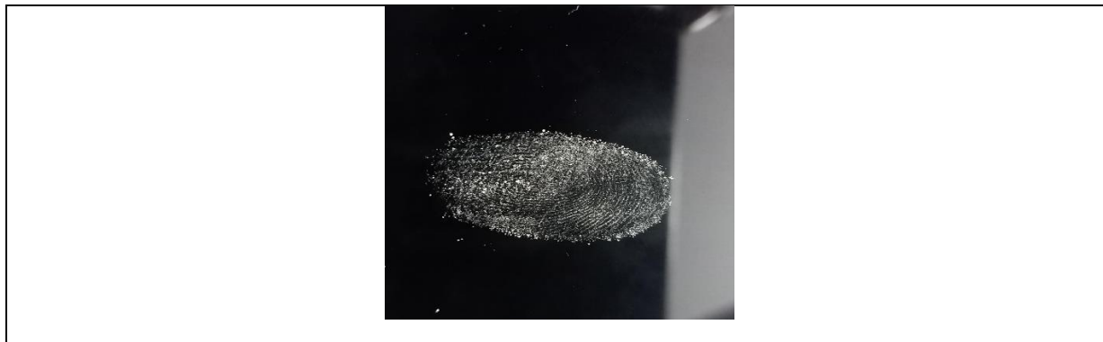
Figure 7: Development of Latent Fingerprint with the help of medicine powder on surface of mobile phone
