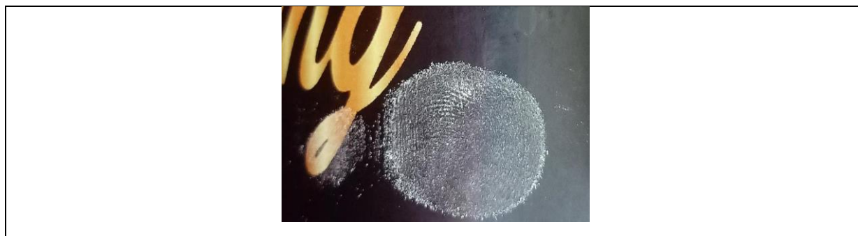
Figure 2: Development of Latent Fingerprint with the help of medicine powder on Coffee Mug Surface
