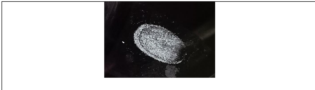
Figure 3: Development of Latent Fingerprint with the help of medicine powder on Induction Cooker Surface.
